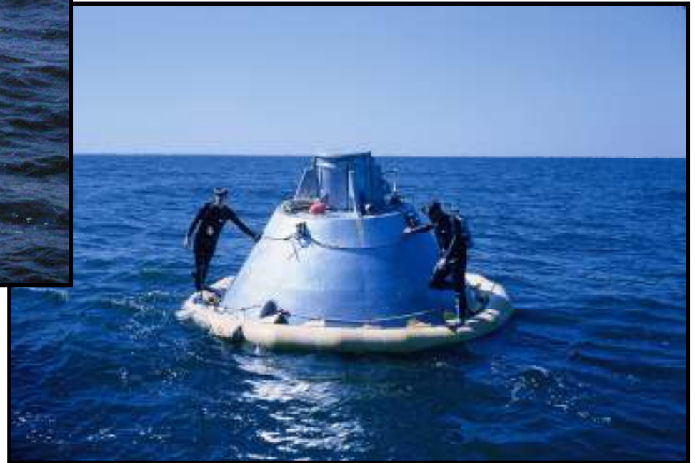
Flotation Collar on BP-1101
