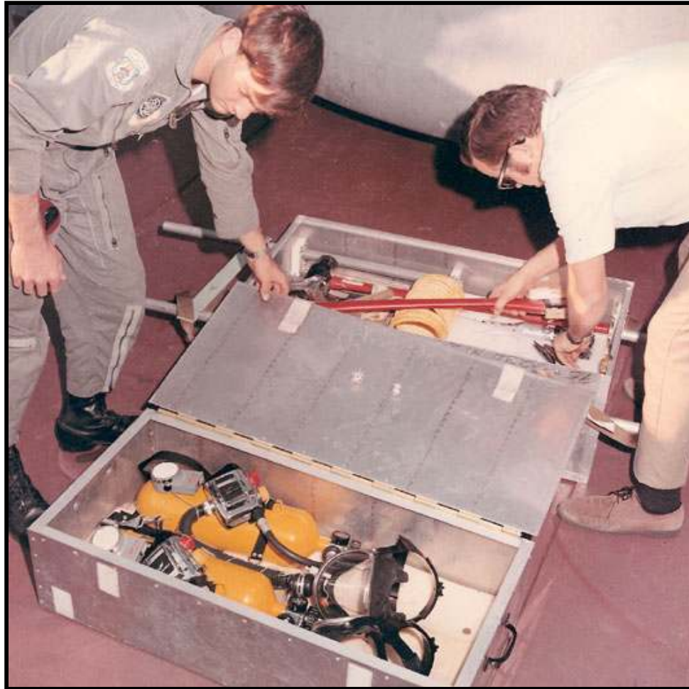
Jammed Hatch Kit (JHK) with emergency access tools and crew breathing equipment in two-part aluminum case with stowable litter handles and lifting sling (not pictured is portable ventilator) for Apollo 13 at KSC in April 1970
