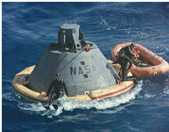
1200 series boilerplate during recovery exercise in Atlantic on 22 nd February 1966
