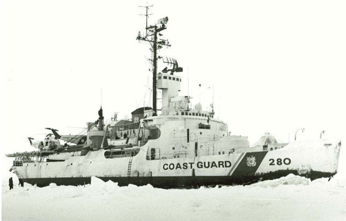
Southwind stuck in the ice where she encountered a polar bear christened Rodney by the crew. Eventually freed herself by rocking the hull to and fro by transferring fuel from port to starboard tanks. Note the boilerplate on the foredeck.
