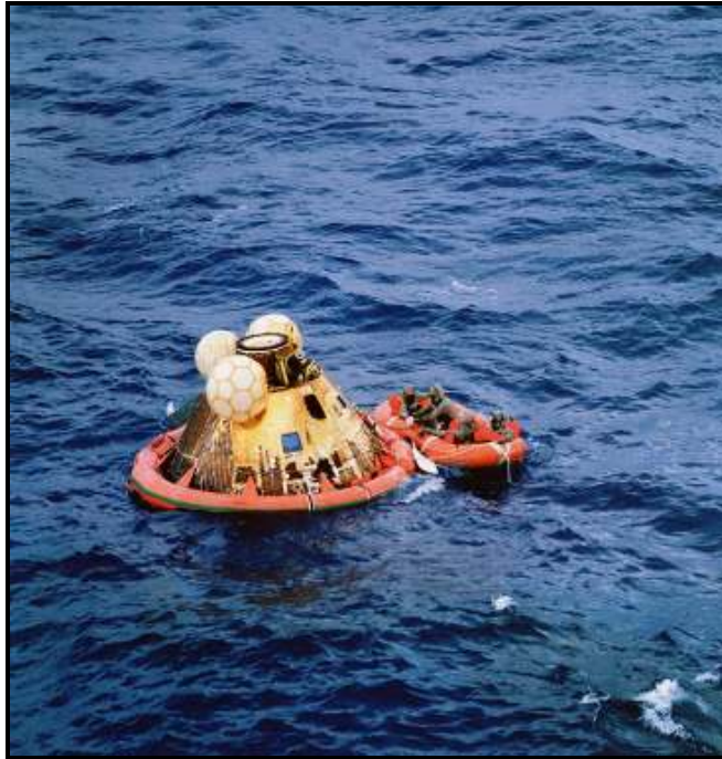
Photo #15: Apollo 11 Block II Command Module post-splashdown with uprighting bags inflated and flotation collar installed. Apollo 11 crewmen Armstrong, Aldrin, and Collins and a Navy UDT swimmer in raft in their biological isolation garments are awaiting helicopter pickup for transport to U.S.S. Hornet, prime recovery ship for the historic Apollo 11 lunar landing mission on July 24, 1969 (Photo Credit: NASA S-69-21698).
