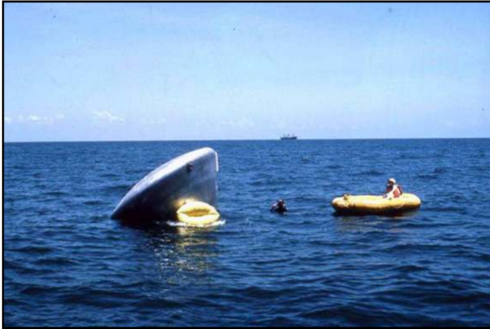
Photo #7: Mid-1965 (est.) photo is Block I BP-1101 in inverted Stable II position with uprighting bag inflating during unmanned Apollo Block I uprighting system test in Gulf of Mexico (Photo Credit: Paul T. Chaput)
