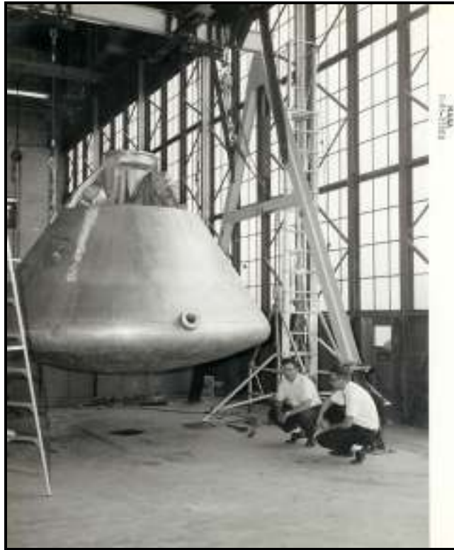
Photo #1: Test setup for initial Block I BP-1101 weight & CG measurement in April 1965. NASA test conductor Ed O'Briant on left, NASA project engineer Coye Mac Jones on right. (Photo Credit: NASA S-65-35838).
