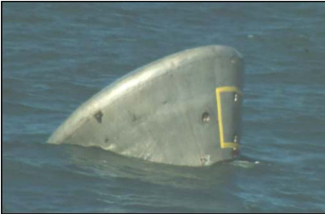
Photo #11: Block II BP-1101A inverted Stable II during unmanned Apollo Block II uprighting system +y bag failure test test in 1967 in Gulf of Mexico (Photo Credit: Still from NASA FR-S67-008 DVD).
