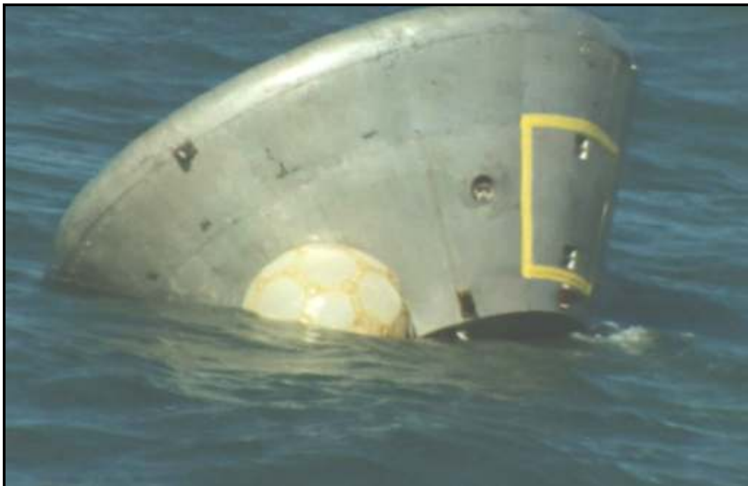
Photo #12: Block II BP-1101A inverted Stable II during unmanned Apollo Block II uprighting system +y bag failure test test in 1967 in Gulf of Mexico (Photo Credit: Still from NASA FR-S67-008 DVD).
