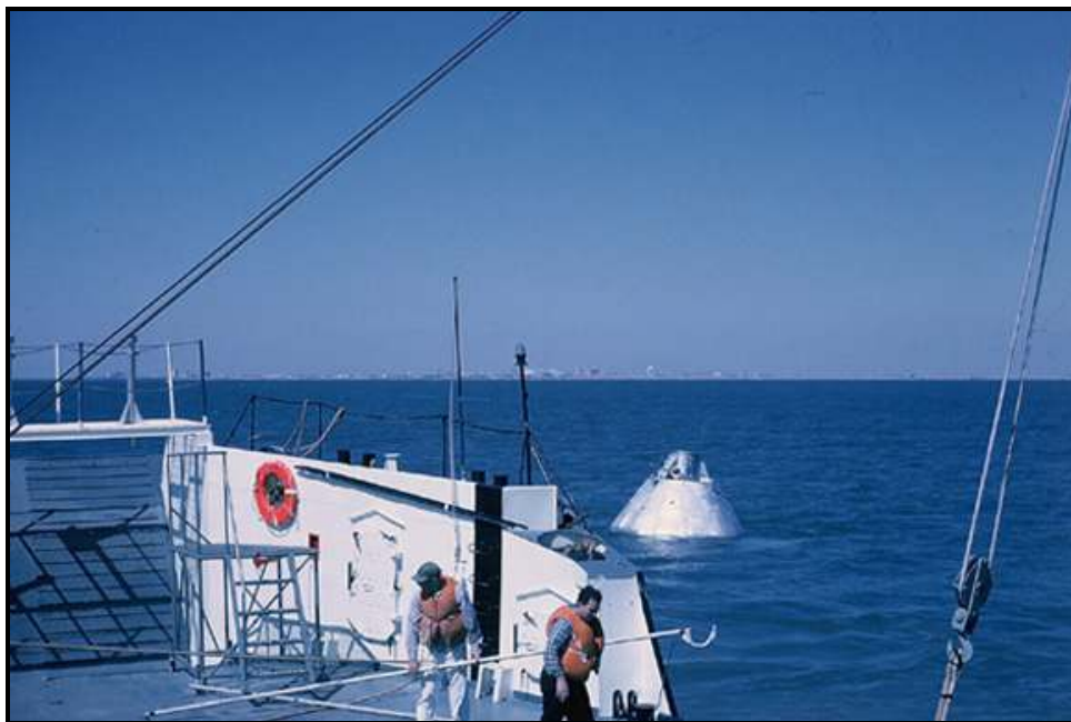
Photo #4: Block I BP-1101 Apollo boilerplate deployed for early Apollo flotation collar test in April 1965 in Gulf of Mexico with Galveston, Texas on horizon (Photo Credit: Coye Mac Jones).
