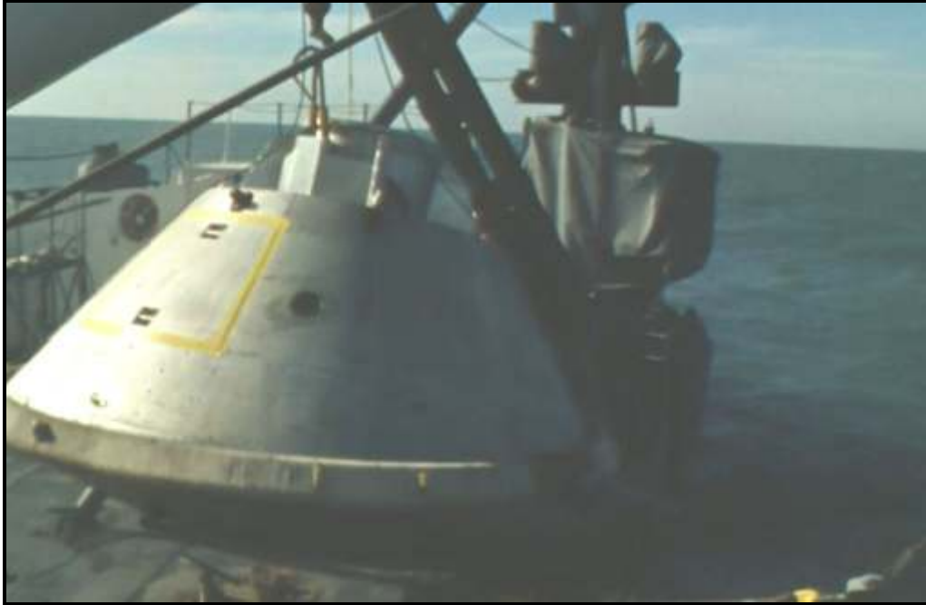
Photo #9: Block II BP-1101A during unmanned Apollo Block II uprighting system test in 1967 onboard MV Retriever in Gulf of Mexico (Photo Credit: Still from NASA FR-S67-008 DVD).
