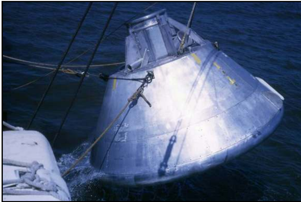
Photo #3: Block I BP-1101 Apollo boilerplate being deployed for early Apollo flotation collar test in April 1965 in Gulf of Mexico (Photo Credit: Paul T. Chaput).
