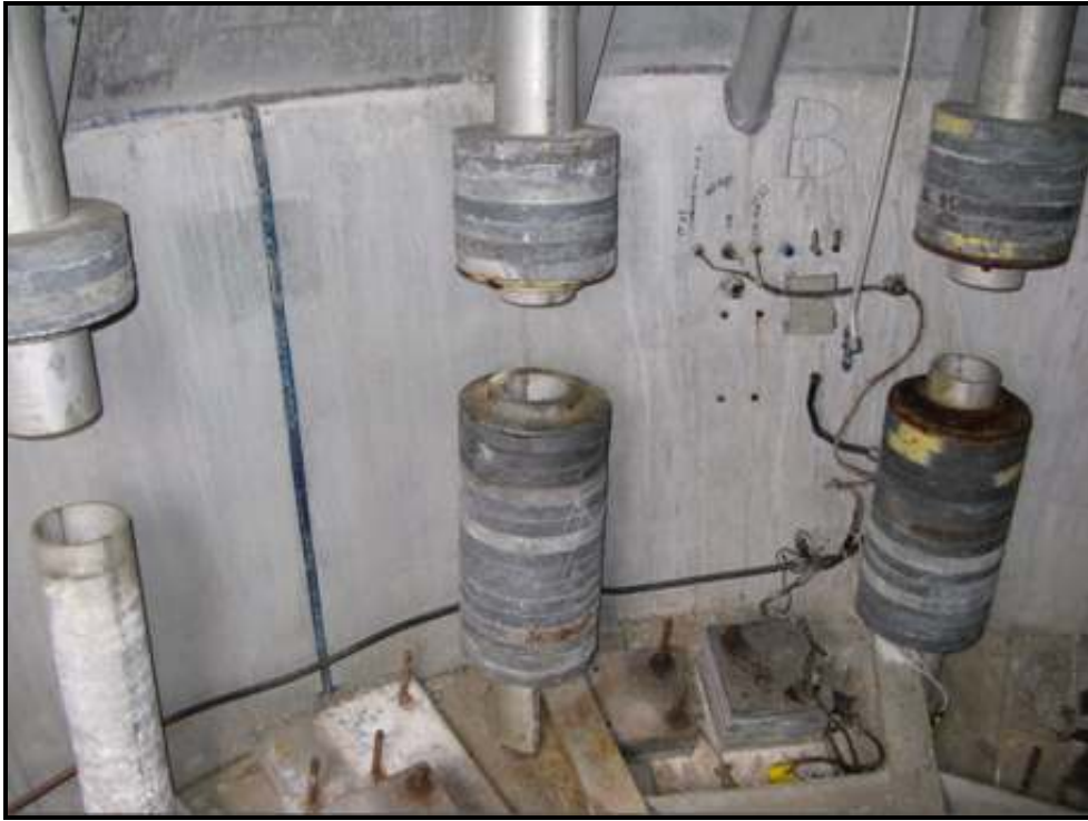
Photo #19: Block II BP-1101A interior showing ballast configuration around circumference during inspection on April 18, 2008 at Wings Museum (Photo Credit: Coye Mac Jones).
