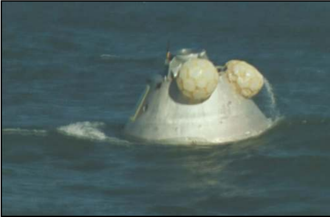
Photo #13: Block II BP-1101A uprighted Stable I during unmanned Apollo Block II uprighting system + y bag failure test in 1967 in Gulf of Mexico (Photo Credit: Still from NASA FR-S67-008 DVD).
