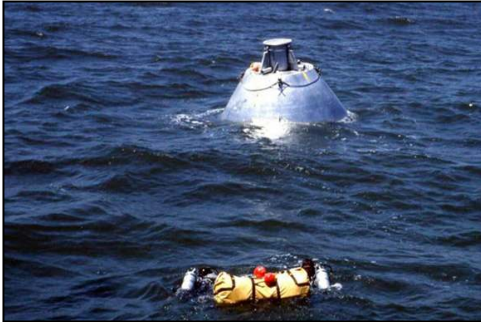
Photo #5: Block I BP-1101 during early Apollo flotation collar test with NASA divers swimming uninflated flotation collar package to BP in April 1965 in Gulf of Mexico (Photo Credit: Paul T. Chaput)
