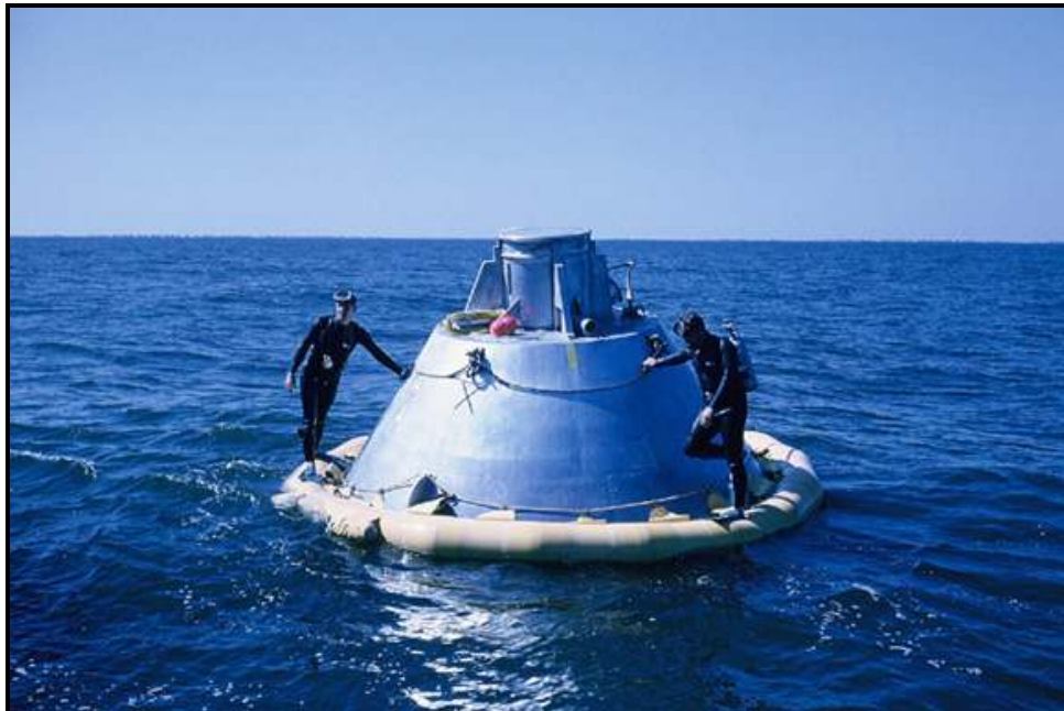
Photo #6: Block I BP-1101 with flotation collar installed/inflated during early Apollo flotation collar test in April 1965 in Gulf of Mexico (Photo Credit: Coye Mac Jones).
