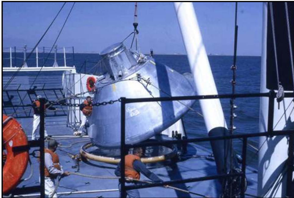
Photo #2: Block I BP-1101 being deployed for early Apollo flotation collar test in April 1965 in Gulf of Mexico from NASA MV Retriever, a converted Army LCU (Photo Credit: Paul T. Chaput).
