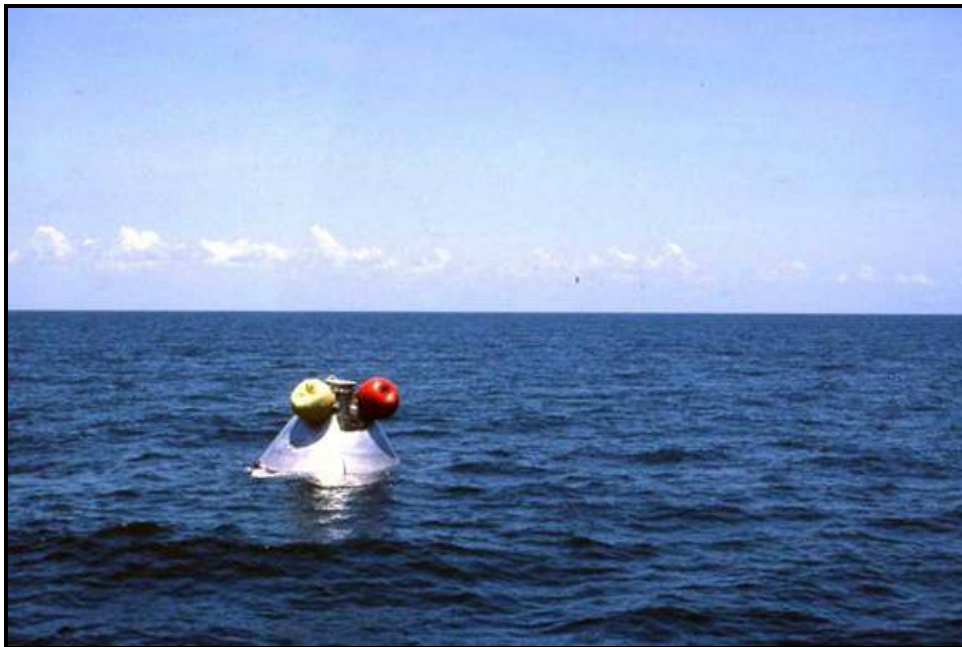
Photo #8: Block I BP-1101 in upright Stable I position with uprighting bags inflated during unmanned Apollo Block I uprighting system test in mid-1965 (est.) in Gulf of Mexico (Photo Credit: Paul T. Chaput).
