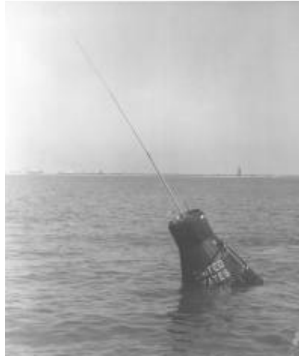
Prototype Mercury Spacecraft with Flight Type Location Aids in Back River
