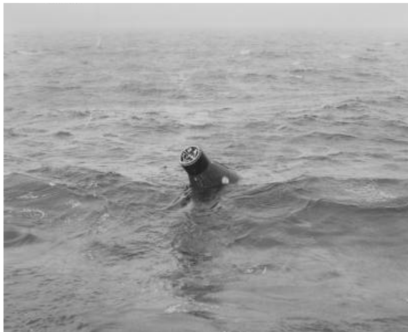
The Ethel H was used to test the final McDonnell landing bag configuration which passed with flying colors
