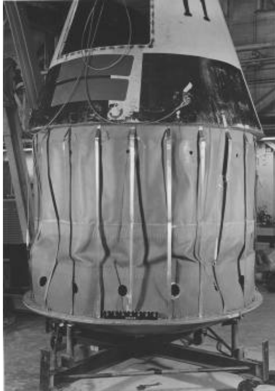
Revised Air Bag Attachment (Note air holes to allow semi-controlled collapse)
