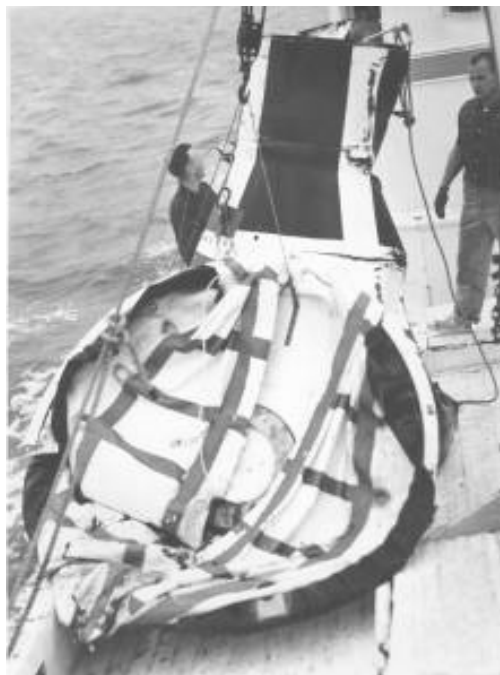
Mercury Boilerplate after Failed Air Bag Seaworthiness Test
