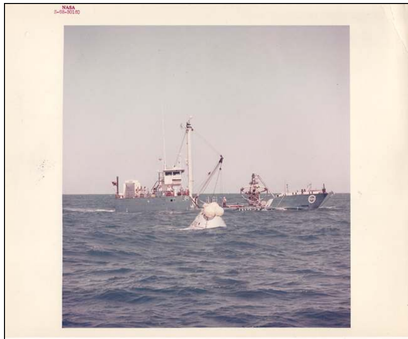
6. CM-007A in Gulf of Mexico next to M/V Retriever during Block II 48-hour manned postlanding systems qualification test with astronaut crew on April 5-7, 1968 (Photo Credit: NASA S-68-30160)
