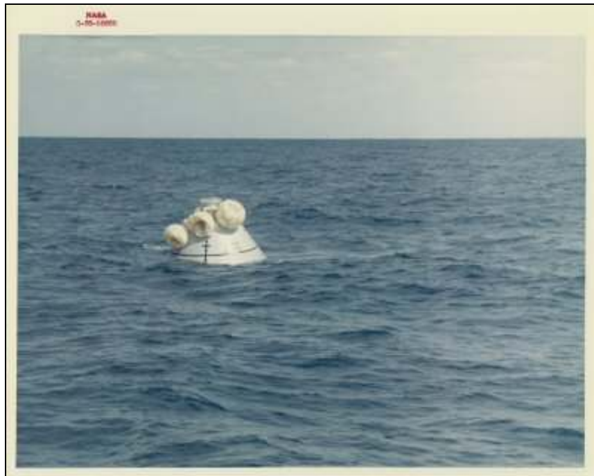
3. CM-007 in Gulf of Mexico during Block I 48-hour manned postlanding systems qualification test on September 30 - October 2, 1966 (Photo Credit: NASA S-66-55668)
